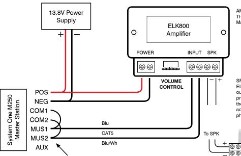
AMPLIFIER LOCATION The amplifier can be installed inside the Master Station
