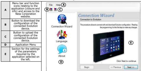
The Evolight software application provides data transfer buttons ( to download the configuration of the connected Evolution device and **=** upload the ongoing configuration.
