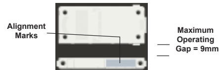
Figure 2. Ness-6021 Mounting Gap and Alignment
