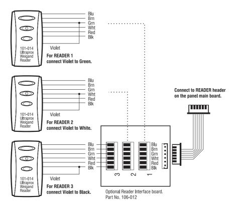
Diagram for connection of up to 3 Ultraprox Weigand Readers to Ness D8x or D16x control panels.
