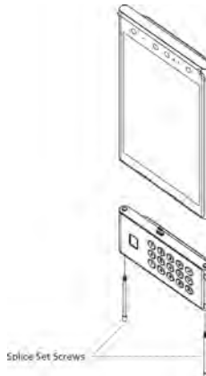
Figure 4-22 Fix Sub Module
