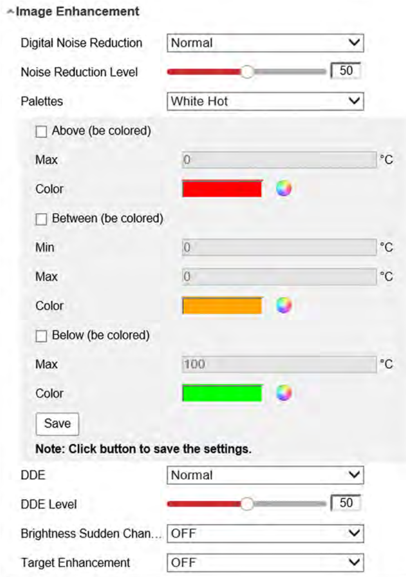
Figure 9-1 Set the Temperature and Color of Target
