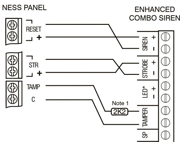
\* Applying 12V to the LED terminals lights one RED LED in the LED array. This may be used as an indicator light driven by an automation output on the control panel.
