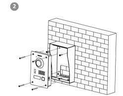
Fix the protective shield on the wall with 4 screws. Install the door station into the protective shield with 4 screws.
