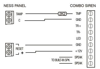
Typical wiring diagram for most Ness control panels. NOTE: Siren timer is controlled by the RESET output from the Ness panel.
