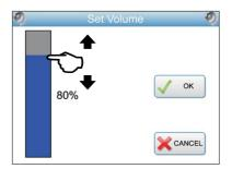
Slide your finger along the Volume slider to adjust the beep volume from 1% to 100%. The volume cannot be set to zero.
