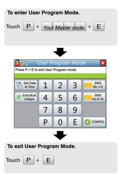
The panel will automatically exit Program Mode if the keypad is inactive for 4 minutes.
