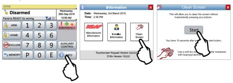
Step 4. The touch screen will be disabled for 10 seconds. Clean the bare screen or the protective film using a soft dry cloth or a cloth moistened with Isopropyl Alcohol.
