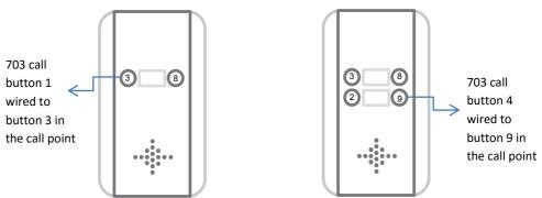
Please note the position of the buttons on the above panel options. For example, if you have a 2 button panel, you will be wiring call buttons 3 and 8. For a 4 button panel, the corresponding button locations are 2, 3, 8 and 9.
