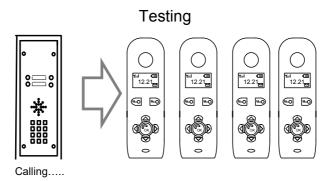
Answer the call on any handset by pressing , and check for good 2 way speech. Adjust volume while on a call with up and down arrow buttons on the handset and press the same button again to end the call. The gate/door release button can be pressed at any time, either while on or off a call. The relay on the transmitter should then pulse on for 4 seconds.
