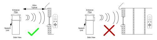
Tip: For longer range installations, locate the handset close to the front of the property, near a window if possible. Concrete walls can reduce the open air range of 350 metres by 30-50% per wall
