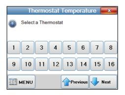
To view the Thermostat temperatures press the "Thermostat Temperature" option from the main menu screen. Then select the Thermostat address which will in return display the temperature
