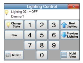
In "Single View" mode, the lighting number can be selected with the numeric buttons. Next Lighting and Previous Lighting buttons will move through lighting items that programmed with show enabled.
