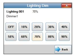
The lighting number, lighting name and current dim level is displayed at the top of the screen.
