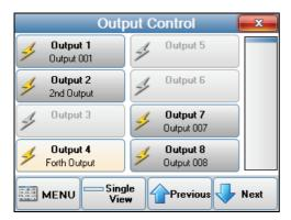
8 output buttons are displayed on the screen at once with each output button displaying the output number and output name.
