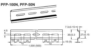
It is recommended to use a panel 1.6 to 2.0 mm thick.
