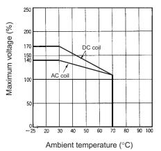
**Note:** The maximum voltage refers to the maximum value in a varying range of operating power voltage, not a continuous voltage.
