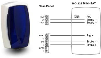
MINI-SAT WIRING TO NESS PANELS
